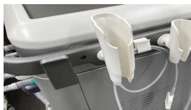
Figure 3.0-11: Location of ground pad cradle
