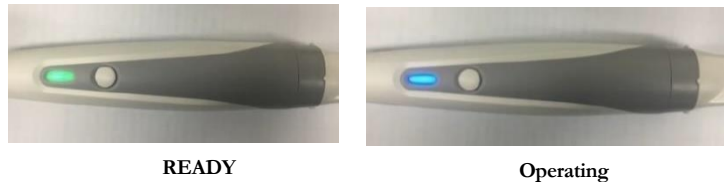
Figure 4.0-14: LED is green in READY mode and blue when operating.
